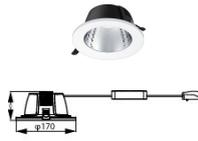
Cut-out hole diameter - Ø150mm
